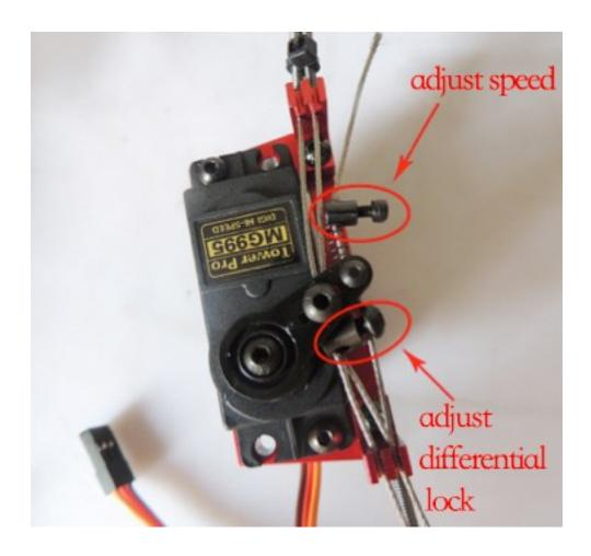
Adjustments when you can't switch to 2-speed differential lock well:
